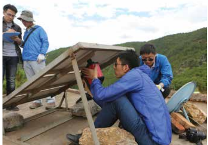
The technical team tested the old modules using an FTIR spectrometer and found they were all based on DuPont™ Tedlar® PVF films.
