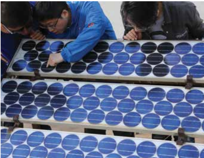
Mono-crystalline modules in use for more than 20 years remain in excellent condition.
