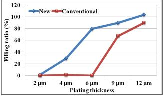
Figure 6 Filing ratio as a function of copper deposition thickness at 1.5 ASD
