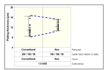
Figure 3 Deposition uniformity of conventional product and new product (12 μm target thickness)
