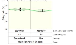
Figure 4 Via-filling performance of conventional chemistry and new chemistry ( $12 \mu m$  target thickness)
