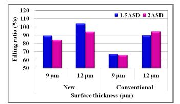
Figure 8 Filing ratio as function of copper deposition thickness and current density
