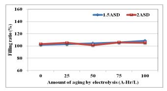
Figure 9 Via-filling performance as a function of aging
