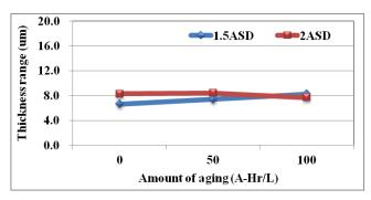
Figure 10 Deposition uniformity as a function of aging
