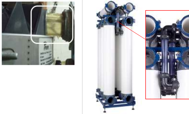
Figure 11.4-3 - Monitoring and ensuring error-free operation of the assembled rack with the help of an integrated transparent pipe on the feed side (in the dizzer® XL Series for Open Platform - left) and on the filtrate side (in the T-Rack® 3.0. and T-Rack® 3.0 S Series - right)
